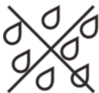
Lamp to be used in dry conditions or in a luminaire that provides protection
