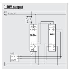
In this mode electronic ballast and transformers with a 1-10V interface up to a total control current of 40mA can be controlled when connected to an universal dimmer switch EUD12D or MFZ12PMD. The EUD12D or the MFZ12PMD is controlled with pushbuttons at the universal control voltage input locally or centrally. The SUD12 converts the dimmer signals from Y1/Y2 to the 1-10V output 0/Q1 for the interface.
