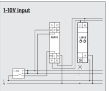
In this mode the output of a 1-10V controller can be converted at A1/0 into a direct dimming function when connected to a capacity enhancer LUD12 at terminals X1/X2. The closing operation and the opening operation is also carried out externally at L of the SUD12. **The rotary switch of the LUD12 must be adjusted to the setting 🌣 (additional lamps).**
