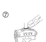
Cut off the cable screen braid right up to the cable fix.
