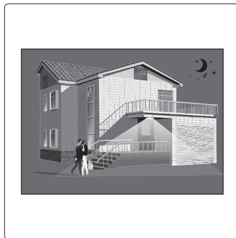
With insufficient ambient light, the sensor switches on the lamp when motion is detected.
