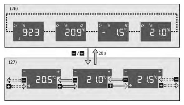
picture 9: Basic setpoint shift using display buttons
