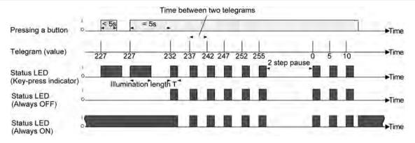
picture 24: Example of value adjustment with value range overflow
