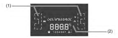
picture 49: Device display and display buttons
