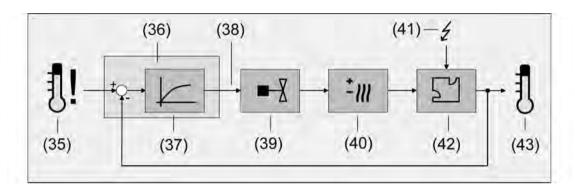
picture 27: Controlled system of single-room temperature control
