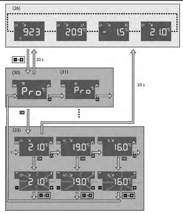
picture 13: Submenu for changing the setpoint temperatures
