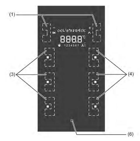
picture 14: Button arrangement (using the example of the triple display variant)
