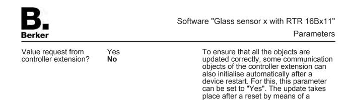
ValueRead telegram to the room temperature controller. The controller must answer the request with a ValueResponse telegram.
