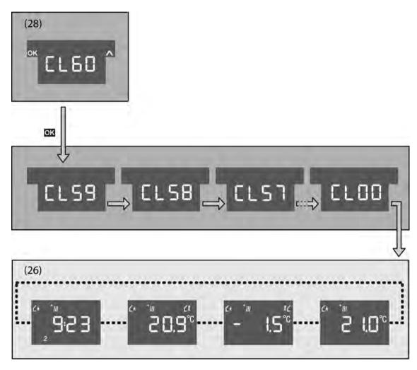
picture 11: Submenu of the cleaning function
