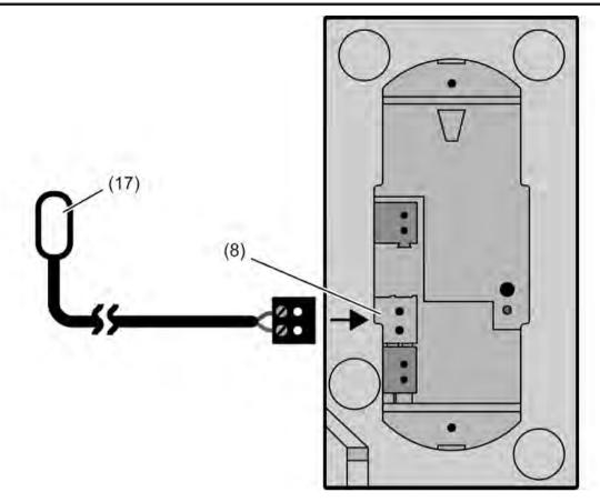
picture 48: Connection for wired temperature/remote sensor
