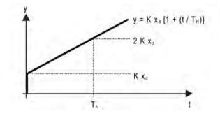
picture 34: Function of the command value of a PI controller
