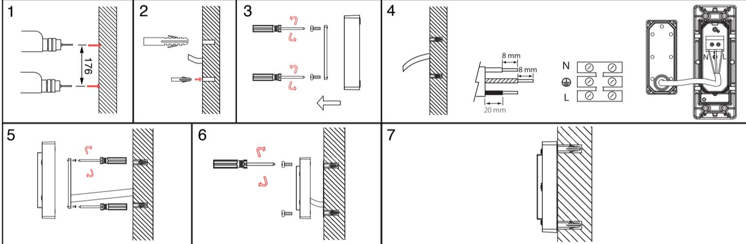
Upaosennus | Infäld montage | Süvispaigaldus | Recessed mounting
