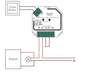
Note: Please follow the detailed wiring diagram of corresponding 2-wire dimmer or switch.
