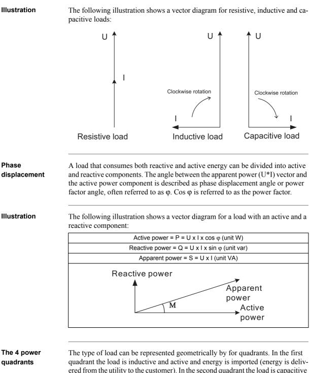
quadrant the load is inductive and active and energy is imported (energy is delivered from the utility to the customer). In the second quadrant the load is capacitive and active energy is exported and reactive energy is imported. In the third quadrant the load is inductive and active and reactive energy is exported. In the last quadrant the load is capacitive and active energy is imported and reactive energy exported.
