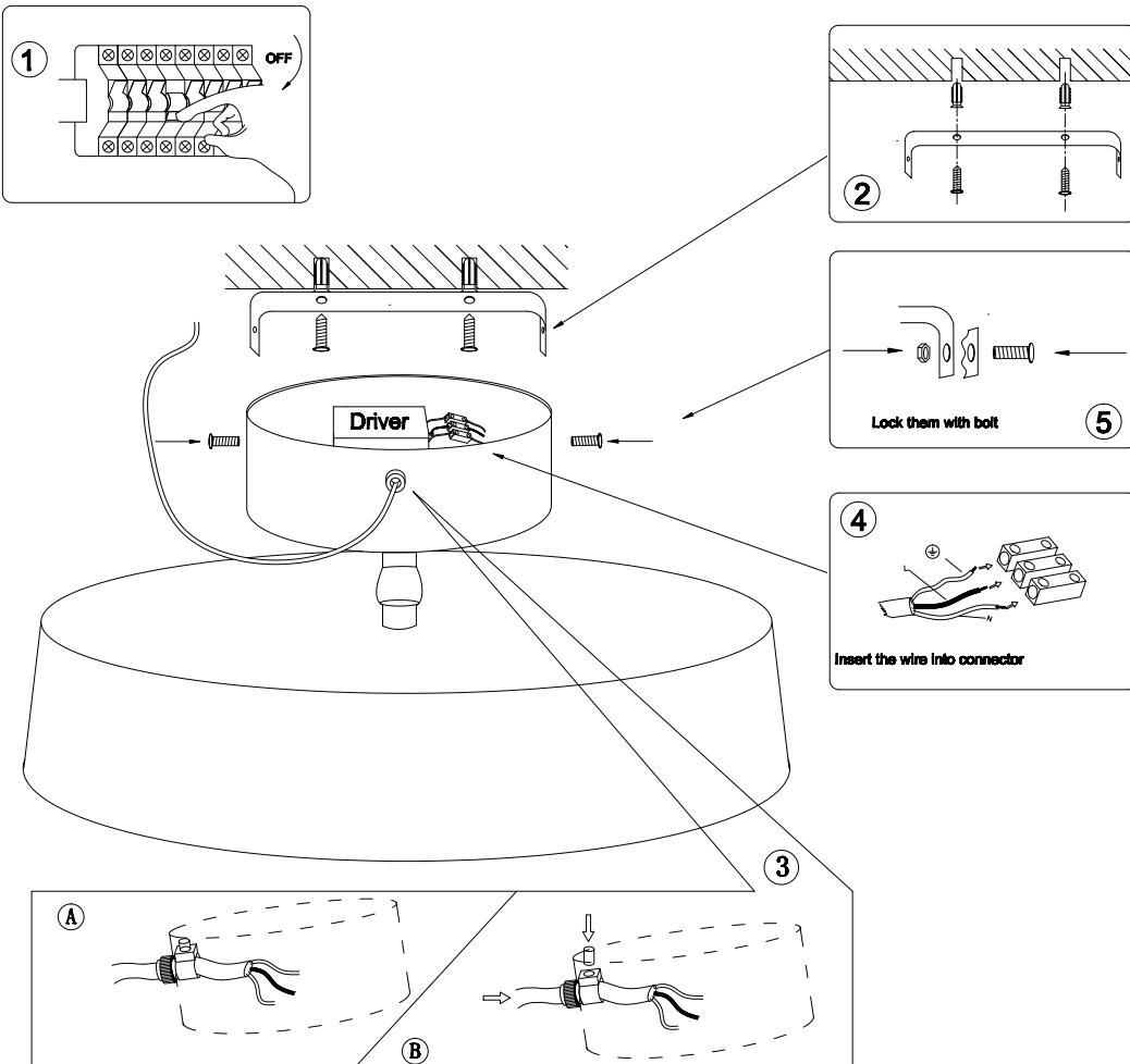
Insert the wire into the canopy hole, and tighten the screw when the cable have been inserted the block terminal.
