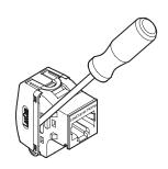
Snap off the cap by means of a screwdriver.
