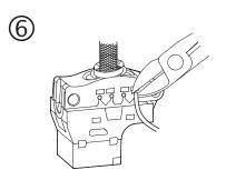
Cut off the conductors right up to the stuffercap (max 1 mm).
