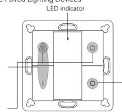
Step 3: Short press 5 times continuously to clear all bound lighting devices . LED indicator flashes 4 times for successful unbinding.
