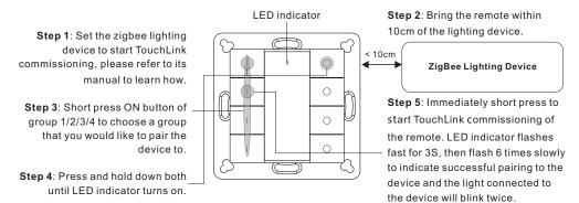
Note: 1) Directly TouchLink (both not added to a ZigBee network), please first factory reset both the remote and device, each remote can link with max. 30 devices, please make sure the first linked device is always powered on when touchlink the remote with 2nd device and more devices.
