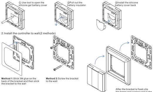
the frame and control part to the bracket in sequence
