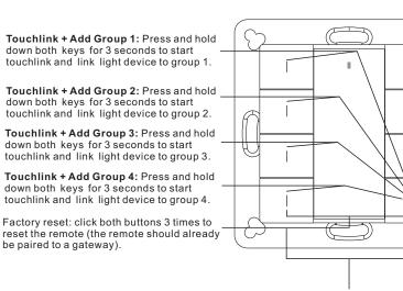
Network pairing mode: click both buttons 3 times to set the remote into network pairing mode (the remote should not belong to any gateway network).
